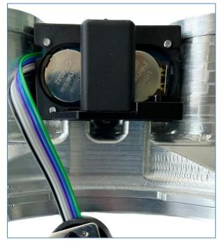
• Open underwater housing. Using hex wrench unscrew 2 bolts from vertical plastic podium (camera support) bottom side. Delete the podium from the housing.
