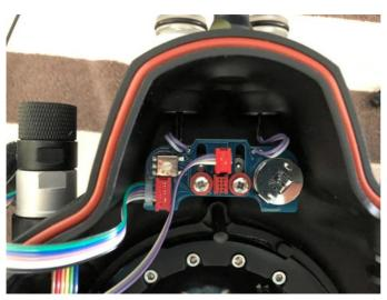
• Insert batteries into TTL-Converter. Before installation check that "plus" terminal of each battery is in Up position.
