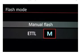
In such Manual mode also becomes available flash output level scale in submenu. User can adjust flash output level by camera wheel, looking to this menu scale (or looking to camera service screen):
