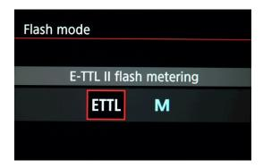
During the initial tests, dependently of concrete camera, strobes condition, batteries etc., photographer should set small constant (+/-) correction to TTL Flash exposure control. Pay attention on this.
