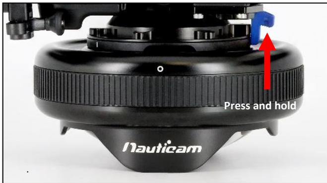
3. Press and hold the BLUE lens release button and then turn the lens count-clockwise.
