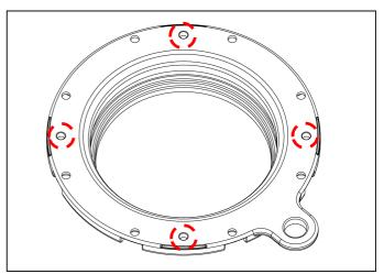
Locate the 4 small sockets in the M67 ring. Align with the 4 positioning pins on the WWL-1 and place it on top.
