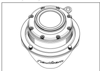
Secure the mounting ring by tightening the eight screws.
