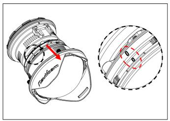
Remove the lens when "I" mark on the lens aligns with the "I" mark on the converter.
