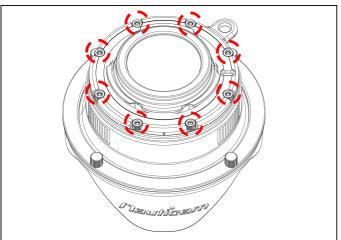
Remove the 8x screws from the back of the lens.
