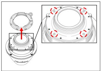
Remove the bayonet mounting ring. Note that there are 4x small black cylindrical positioning pins. All 4 pins should be remain in the back of the lens.
