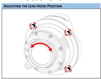
To adjust the position of the lens hood, slightly loosen the four thumb screws as indicated above (one is not visible from the image). Turn the hood to the desired position and secure by tightening the four thumb screws.
