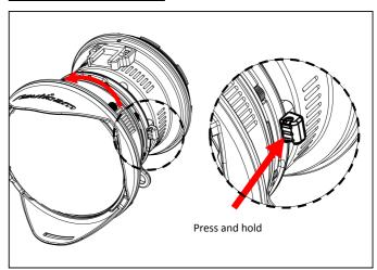
Press and hold the RED lens release button and then turn the lens anticlockwise.
