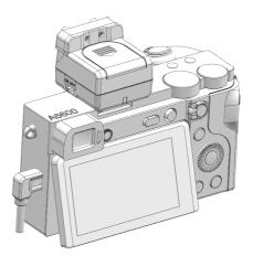
Align the flash trigger hotshoe connector to the camera hotshoe and slide in until it cannot go in any further. Test the flash trigger by pressing the shutter release button of the camera, the LEDs in the front should turn on instantaneously. To detach the flash trigger from the camera, press and hold the Unlock button and slide it out.
