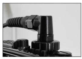
4. Then, tighten the HDMI 2.0 cable by turning the threaded working ring
