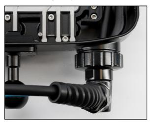
3. Then, tighten the HDMI 2.0 cable by turning the threaded working ring.
