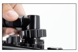
Gently push the cable into the M28 port opening of the housing, until it cannot go in any further.
