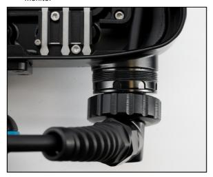
Align and plug the HDMI 2.0 cable in the M28 port opening.
