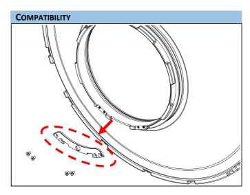
This port is backwards compatible with other N120 extension rings. A user installable locking tab is pre-installed for this purpose.
