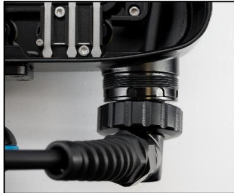
2. Align and plug the HDMI 2.0 cable in the M28 port opening. Gently push the cable into the M28 port opening until it cannot go in any further.
