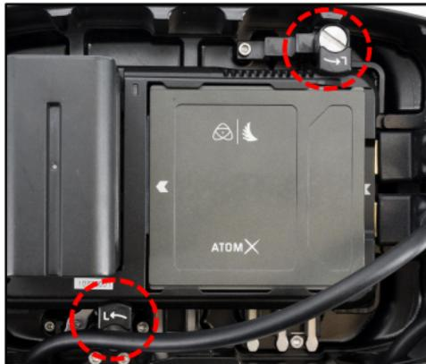
2. Secure the monitor by turning the two locking levers towards the monitor as shown.
