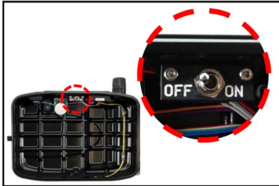
2. Switch the alarm on. The LED light will flash blue once and turn blue for five seconds indicating the battery is normal. Then it goes into flashing blue light standby mode.
