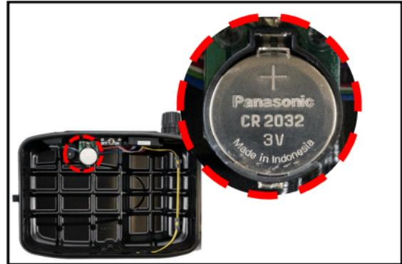
1. Ensure that remove an insulation film before install a battery. Then install the battery provided into the battery compartment on the circuit board inside the housing.
