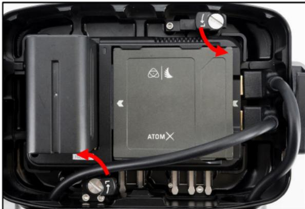
1. Before mounting the camera, connect HDMI 2.0 cables (IN and OUT) to the camera's HDMI connectors accordingly.
