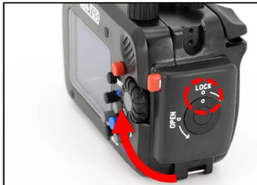
2. Turn the housing lock clockwise for 270°, until the lock reaches the "lock" position as shown. Confirm that the white indicator line on the safety button is visible.
