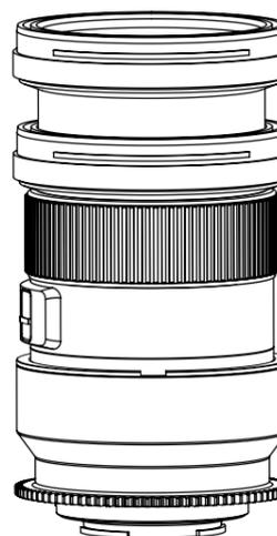
3. The tightness between the both gears and the lens can be adjusted by removing or adding rubber grips on either sides of the plastic C-ring, spare rubber grips are included in the package.
