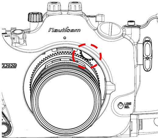
1. The SSF2470-Z Zoom Gear can be controlled by zoom/focus knob of the housing.
