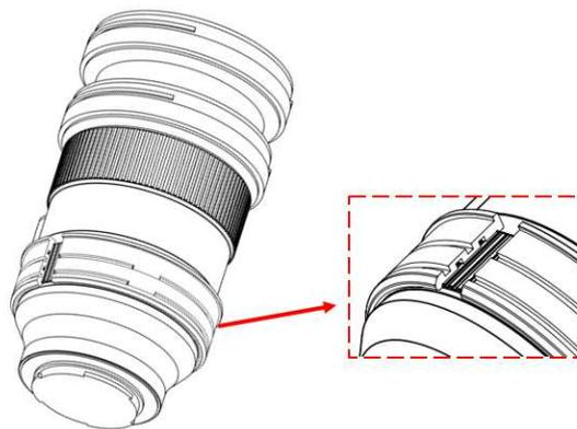
1. Insert the plastic C-ring for zoom gear as shown and place it over the lens
