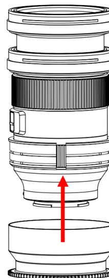
2. Insert the SSF2470-Z Zoom Gear on the plastic C-ring until it reaches the flange of the plastic C-ring.
