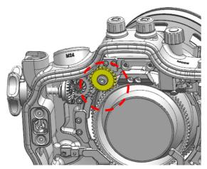
1. The SFE28135-Z Zoom gear can be controlled by zoom/focus knob of the housing.
