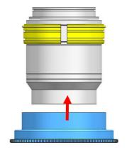
Insert the SE2870-F\_Focus Gear on the plastic C-ring until it reaches the flange of the plastic C-ring.
