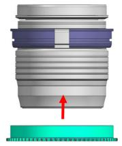
2. Insert the O1245-F Focus gear on the plastic C-ring until it reaches the flange of the plastic C-ring.
