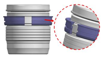
Insert the plastic C-ring for Zoom as shown and place it over the lens
