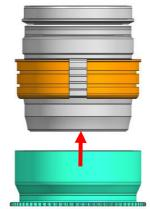
2. Insert the O1245-Z Zoom Gear on the plastic C-ring until it reaches the flange of the plastic C-ring.
