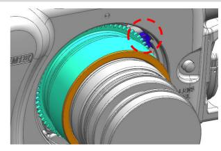
The O1245-Z Zoom Gear can be controlled by zoom/focus knob of the housing.
