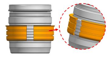
1. Insert the plastic C-ring as shown and place it over the lens
