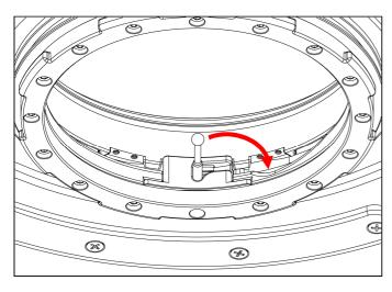
5. To lock the extension ring, push the locking pin inwards.
