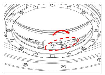
6. Turn the locking device sideways into the recess. Ensure that the locking device is secured inside the recess and the extension ring is securely locked with the port.
