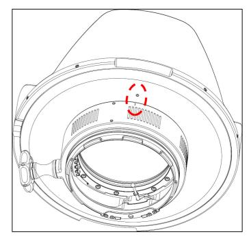
2. Align the "I" mark on the extension ring with the WHITE dot on the port.
