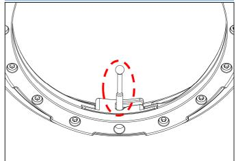
1. Confirm that the extension ring is unlocked, with the locking pin pointing upwards as shown.
