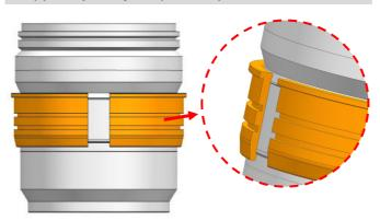
Insert the plastic C-ring as shown and place it over the lens 1.
