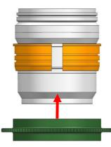
2 Insert the PL2060-Z Zoom Gear on the plastic C-ring until it reaches the flange of the plastic C-ring.
