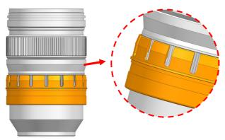
1. Insert the plastic ring as shown and place it over the lens.
