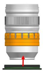
Insert the PL2470-Z Zoom Gear on the plastic ring until it reaches the flange of the plastic ring.
