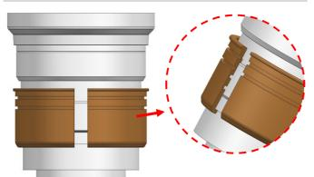
1. Insert the plastic C-ring as shown and place it over the lens
