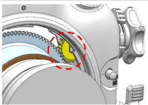
1. The CT1120-Z Zoom Gear can be controlled by zoom/focus knob of the housing.
