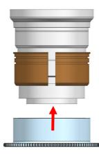
2. Insert the CT1120-Z Zoom Gear on the plastic C-ring until it reaches the flange of the plastic C-ring.
