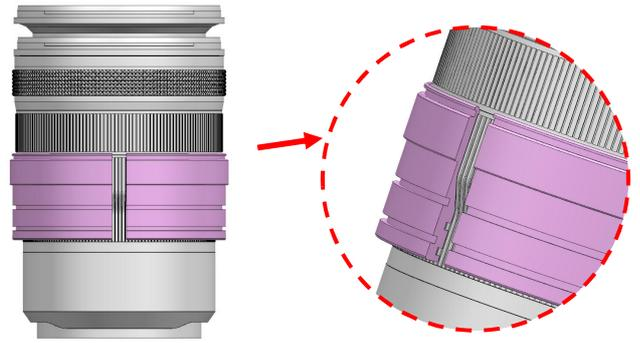
1. Insert the plastic C-ring for zoom as shown and place it over the lens
