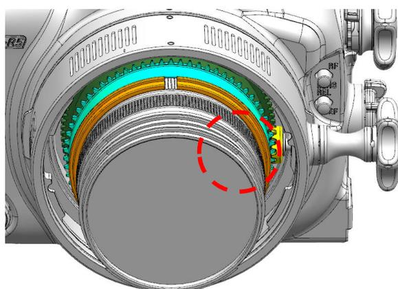
2. The WCR1535-F focus Gear can be controlled through the focus knob of #21235 N120 Extension Ring 35 with Focus Knob.
