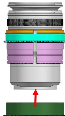
4. Insert the CR1535-Z Zoom gear on the plastic C-ring for zoom until it reaches the flange of the plastic C-ring.
