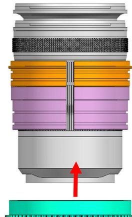
3. Insert the WCR1535-F Focus gear on the plastic C-ring for focus until it reaches the flange of the plastic C-ring.
