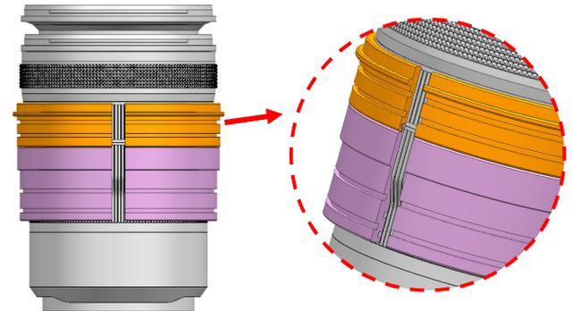
2. Insert the plastic C-ring for focus as shown and place it over the lens, then lock the focus c-ring as shown.
