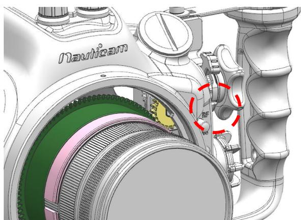
1. The CR1535-Z Zoom gear can be controlled by zoom/focus knob of the housing.
