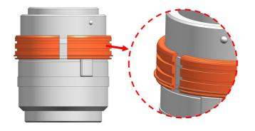
Insert the plastic C-ring for Zoom as shown and place it over the lens
