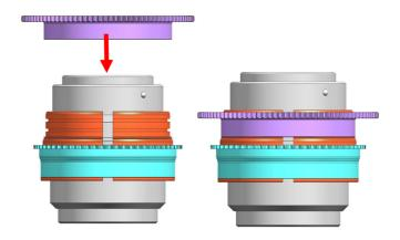
4. Insert the **#19557** C2870f3.5II-Z Zoom gear on the plastic C-ring for Zoom until it reaches the flange of the plastic C-ring.
