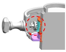
1. The C2870f3.5II-F Focus gear can be controlled through the focus knob of #21230 N120 Extension ring 30 with focus knob.
