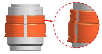
2. Insert the plastic C-ring for Focus as shown and place it over the lens, then lock the zoom c-ring as shown.
