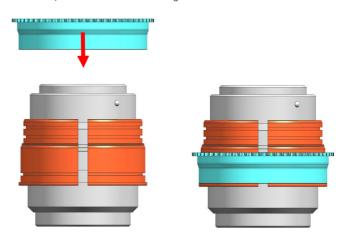
3. Insert the C2870f3.5II-F Focus gear on the plastic C-ring for Focus until it reaches the flange of the plastic C-ring.
