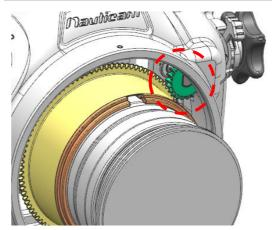
1. The NZ2470f2.8S-Z Zoom Gear can be controlled by zoom/focus knob of the housing.
