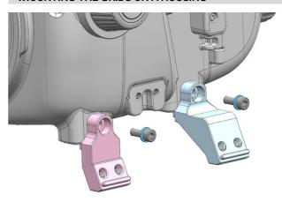
1. Mount the support fixtures on the housing as shown above.
