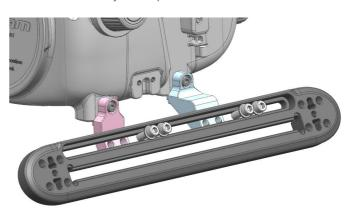
3. Attach a housing skid on the support fixtures as shown above.
