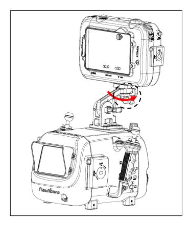
Lift the Rotation lock/release lever to allow the monitor housing moving left and right. Lock it in position by pressing it down with a click sound.
