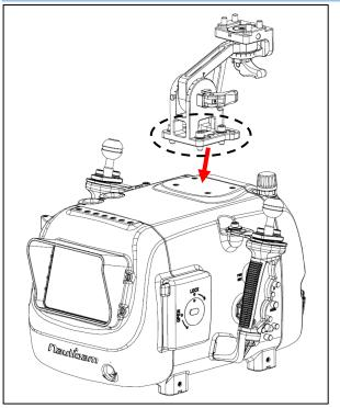
Align the screws on the bottom bracket with cinema housing mounting holes. And fasten it by tight the 4 screws.
