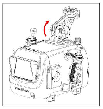
Lift the tilt lock lever to allow the bracket moving up and down. Lock it in position by pressing it down with a click sound.
