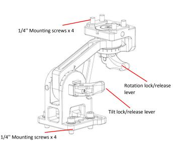
\*The red o-ring comes with each screw on the mounting bracket are for retaining the screws in place. Please remove them before installing the bracket with housings.
