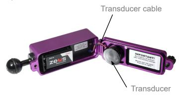
Take care that the transducer cable is not squeezed when closing the lid.
