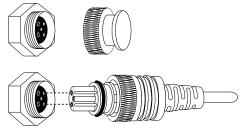
4. Hand-tighten the retaining ring.
