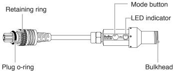
Apply a very thin, even layer of lubricant on all threads, sealing surfaces, and the exposed portion of the plug o-ring. Do not allow lubricant to get into the pins and receptacles of the plug or bulkheads.
