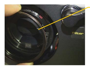
A diopter can be threaded onto the camera directly.
