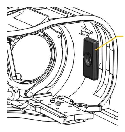
Press the 4 ounce weight on in this location when using the SP34A or FP34A
