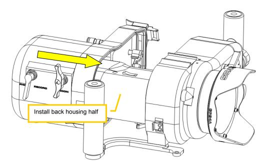
**Carefully inspect the parting line** between front and rear housing. If this line is not even all the way around, remove the back and determine the reason. (O-ring out of place, hand strap interference, etc.) Failure To Do This May Result In A Wet Camera!
