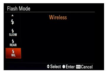
Based on your camera firmware, if "WL" sign doesn't show on the Flash Mode Menu, it can also be found on page 11 of Camera Menu 1. When ON, it will override the flash mode setting menu and the TTL system will operate in Manual Mode only.
