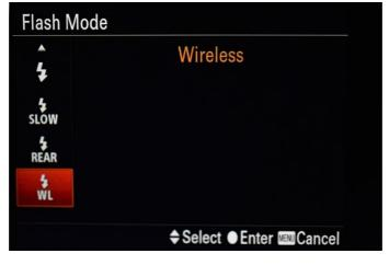
Based on your camera firmware, if "**WL**" sign doesn't show on the Flash Mode Menu, it can also be found on page 11 of Camera Menu 1. When ON, it will override the flash mode setting menu and the TTL system will operate in Manual Mode only.
