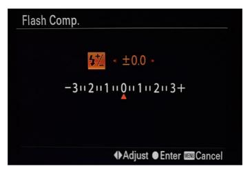
In common case, during the normal operation, the TTL (+/-) flash exposure compensation adjustment is available for underwater photographer through 2 methods:
