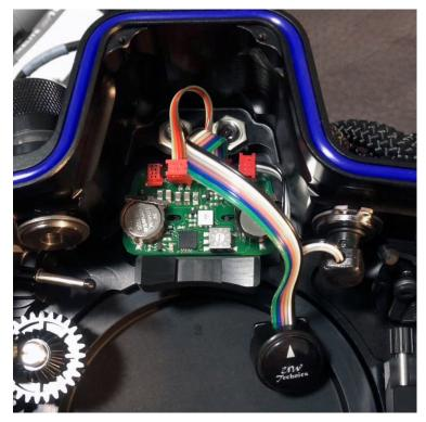
• Replace original optical bulkheads of the housing by special optical bulkheads for LEDs, included with TTL-Converter. Tighten the nuts slightly. Fix the nuts by a drop of paint, to prevent unscrewing for future.
