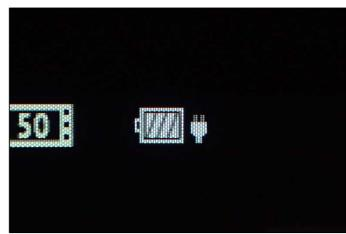
Confirm that the battery pack is active and charging the camera before closing the housing. The battery level icon in the camera will charge to a socket icon when external battery is connected.
