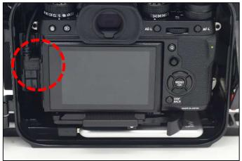
Plug the micro USB cable into the camera's micro UCB port.
