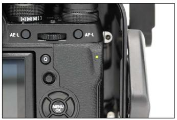
When the battery pack is connected to the camera, the indicator lamp of X-T2 will turn on indicating it is charging the internal battery of X-T2. The lamp will off once the charging is completed.
