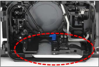
Connect the micro USB cable to the battery pack and slide into the slot at the bottom of the housing as shown.
