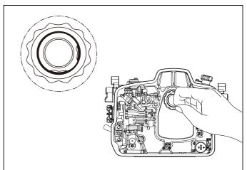
Remove the retainer O-ring of the viewfinder inside the rear half of the housing by making use of the recess on the viewfinder.
