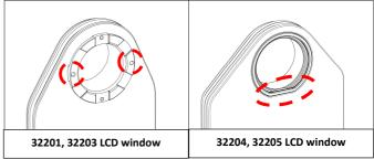
Align the viewfinder's alignment pins/ slot with the holes/ slot of the sleeve in the LCD display window.
