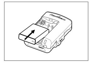
Install the battery. Make sure the +ve and –ve terminals are correctly oriented. Then return the cover to its original position.
