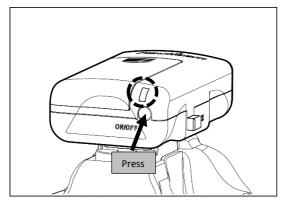
Press and hole the on/off button for at least 1 second to turn on the flash. The power lamp turns on and flash recycling starts. Check that the indicator is lit, when the indicator lights, you can shoot with the flash.
