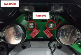
Remove the original LED flash trigger from the housing by unscrewing the two screws as indicated above.
