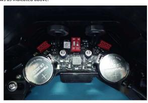
Install the TTL converter and simultaneously insert both LEDs into the optical bulkheads.
