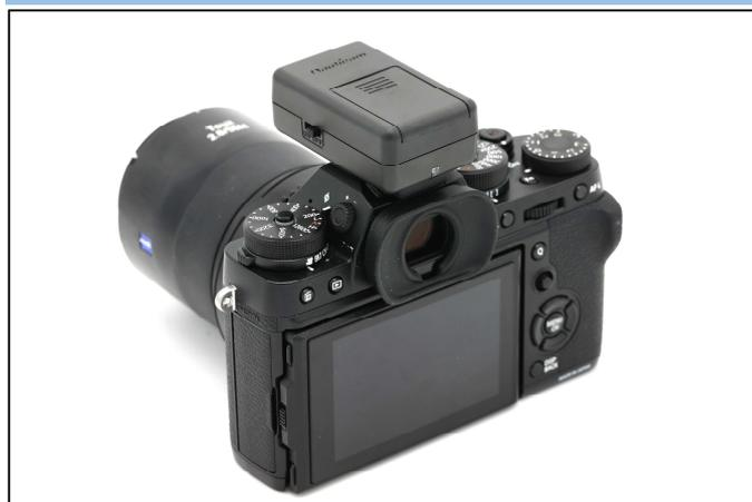
Align the flash trigger hotshoe connector to the camera hotshoe and slide in until it cannot go in any further. Test the flash trigger by pressing the shutter release button of the camera, the LEDs in the front should turn on instantaneously.
