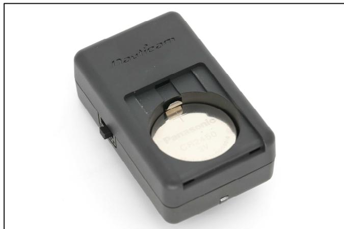
Install the batteries (CR2450 x2pcs) with +ve terminal facing up as shown above. Close the battery compartment cover and then switch the trigger unit on. The indicator will turn green.
