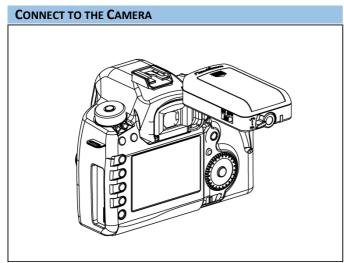
Make sure the locking lever is in "REL" position. Slide the flash trigger hotshoe connector into camera hotshoe until it cannot go in any further.
