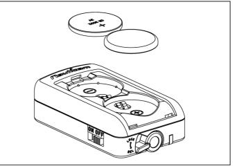
Install the batteries as shown. Please note that the "+" and "-" sign on the battery holders denotes the sides of the batteries facing down.
