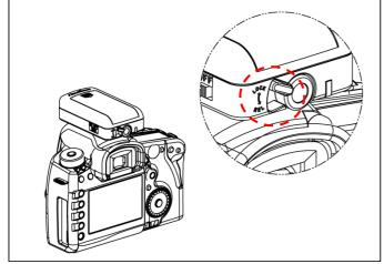
Flip the locking lever to the "LOCK" position to secure the trigger.
