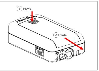
Make sure the On/Off switch is in the OFF position. Remove the batteries compartment cover by sliding it outwards.
