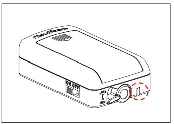
Close the battery cover and then switch the trigger unit on. The indicator will turn green.
