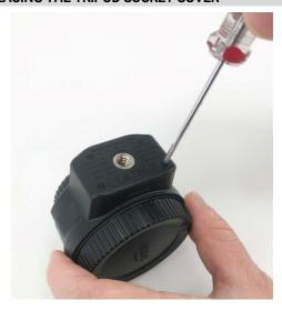
Unscrew 4x screws from FTZ mount adaptor bottom, then remove the original tripod socket cover.
