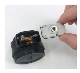
2. Take the metal tripod socket block out
