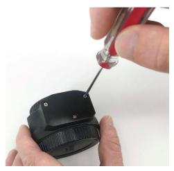
3. Place the tripod socket replacement cover onto the FTZ adapter, and tighten it with the 3x screws provided.
