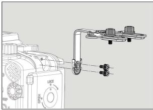
1. Locate the mounting holes on the side/top of the housing and install the handle bracket to the housing as shown. Remove the retaining nuts before mounting the bracket.
