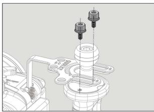
**2.** Attach the tray to the housing and align the bracket to the threaded holes of 71311. Adjust the position of the handle if needed.
