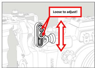
**2.** Loose the two screws as shown until the wheel assembly can freely move vertically. Then adjust the position of the wheel so that it touches on the housing shutter release lever and then tighten it.
