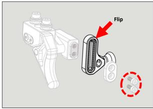
**1.** The position of the wheel can be switched by removing the two screws as indicated and flip the wheel assembly to the preferred position.
