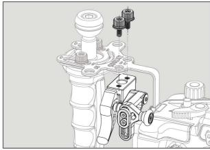
1. Mount the shutter release extension onto the right handle bracket as shown. If the wheel of the shutter release extension is too far or too close the housing, reposition the wheel as instructed in step 1.
