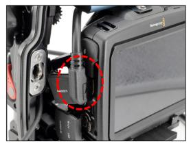
Before locking the camera tray in, connect the HDMI 2.0 cable with the camera's HDMI port.
