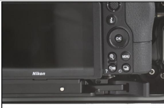
6. If installing the camera with lens and gear attached, Pull down the Zoom/ focus gear disengagement lever before mounting lens (with gears installed) to the camera. Engage the gears by pulling up the lever to the original position. Confirm that the zoom/focus knob operates correctly.
