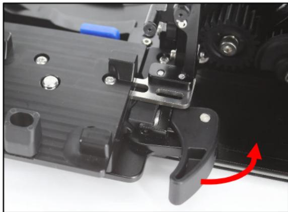
1. Turn the locking lever on the tray of the housing to the “open” position as shown. Then remove the camera saddle from the housing by sliding it outwards.
