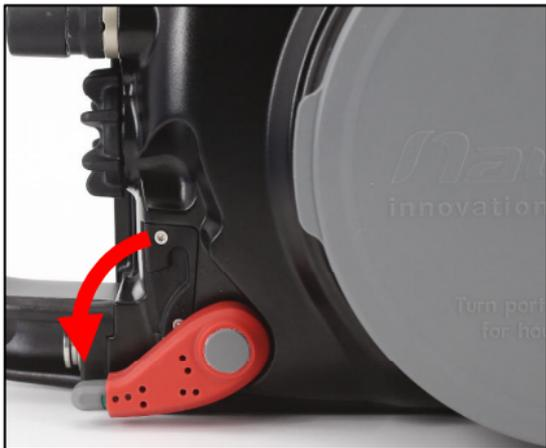
4. Turn the port locking lever to the release position as shown.
