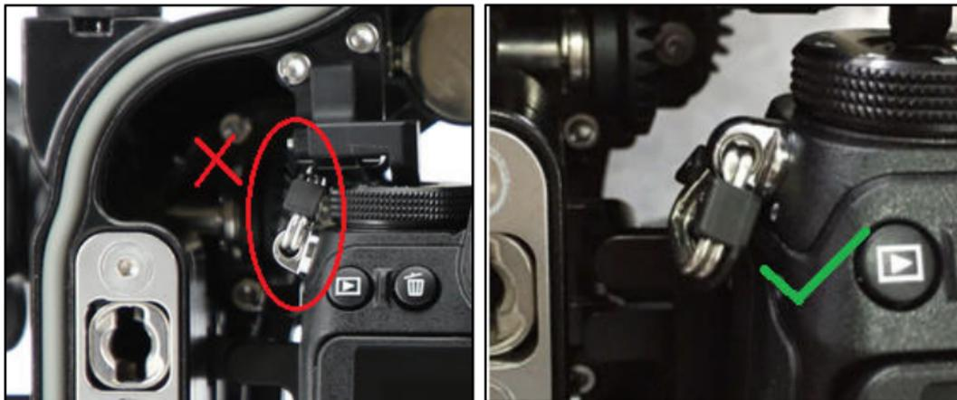
9. The left landyard ring should be placed on the lower position. If not it would interfere with internal part and stop you to lock the housing.
