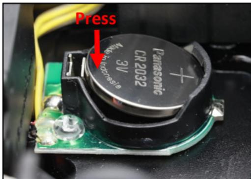
Insert the battery as shown above and then press down the battery.
