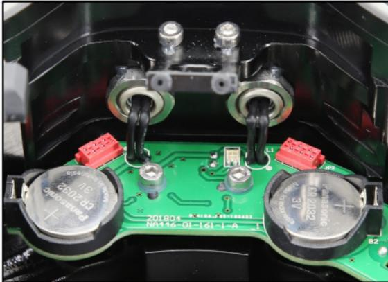
1. Insert the 2x CR2032 batteries into the battery holders. Please noted that the positive terminal should be facing up.
