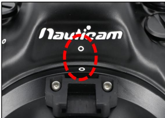
6. Align the Port mounting indices of the port and the housing.
