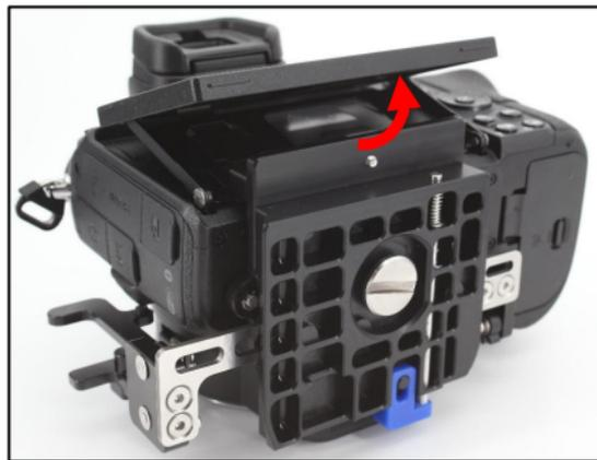
2. Tilt the LCD monitor of the camera upwards, then attach the saddle to the camera by tightening the screw to the tripod socket of the camera.
