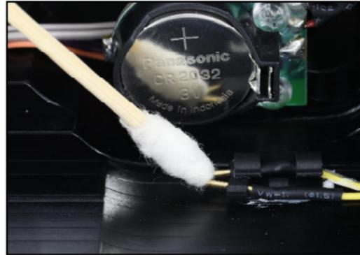
3. Test the alarm by connecting the two wires near the bottom of the housing with a damp cotton bud; the alarm should start giving out a repeating “beep” sound along with a flashing red light. The “beep” sound and the light should keep on going for 5 seconds after the removal of the damp cotton bud.
