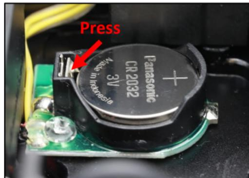
To remove the battery, press the metal plate as indicated and the battery will pop out.
