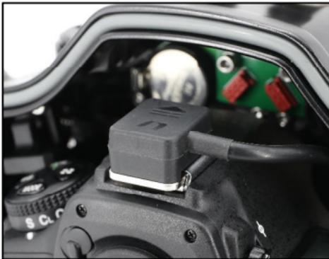
4. Mount the camera by sliding the attached saddle along the rail in the housing until it cannot go in any further.
