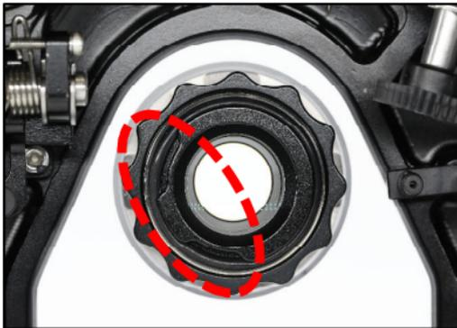
1. Remove the retainer O-ring of the viewfinder inside the rear half of the housing by making use of the recess on the viewfinder.
