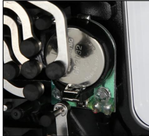
1. Locate and install the battery provided into the battery compartment on the circuit board inside the housing.
