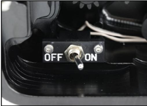
2. Switch the alarm on. The LED light will flash blue once and turn blue for five seconds indicating the battery is normal. Then it goes into flashing blue light standby mode.
