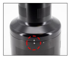
4. Turn the port adaptor clockwise until the "o" mark on the port adaptor aligns with the "o" mark on the extension ring.
