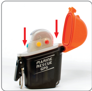
Unscrew two screws on top cap
