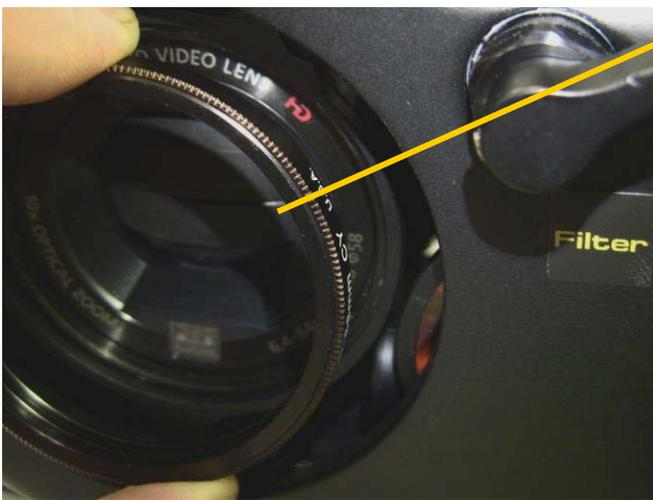
A diopter can be threaded onto the camera directly.
